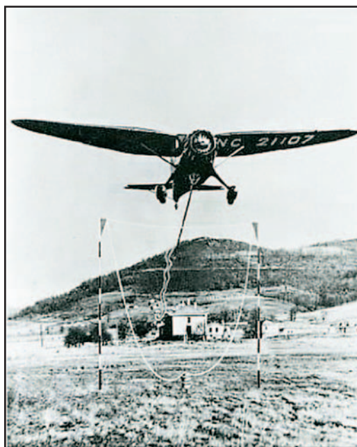
Bizarre but very efficient, the pick-up and delivery system known as "clothesline mail" brought airmail service to small-town America
